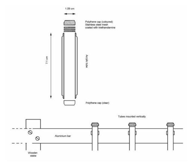
Figure 5. Diffusion tube used for long-term monitoring of nitrogen dioxide and its position in the field
