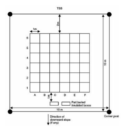
Figure 10. Layout of soil solution sampling area
